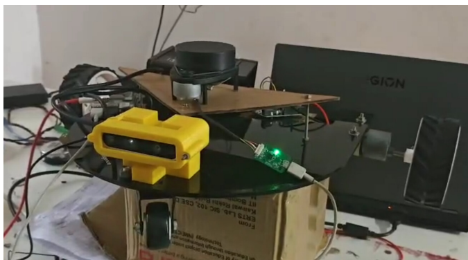
(a) The rig with lidar and depth camera
